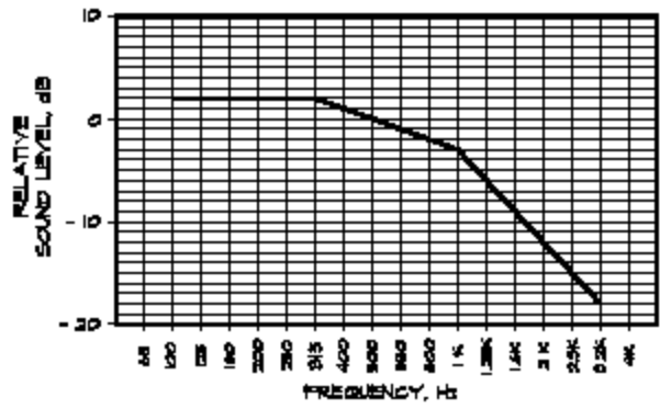
FIGURE 12.8 Reference Contour for Calculating Impact Insulation Class and Other Ratings (ASTM E989, 1989)
